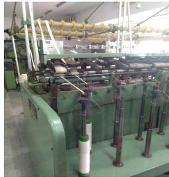
**Figure 5. Roving Process**
