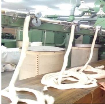
**Figure 4. Drawing Process**
