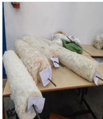
Figure 2. Blended Fiber rolled on the rod
